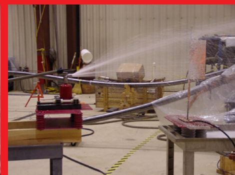
Figure 4. 0.95-L PFE Extinguisher UL 711 (Class C) - Test in Progress
