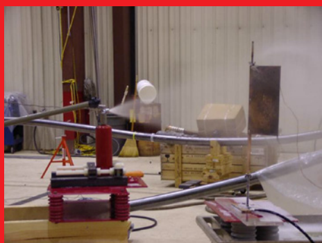
Figure 3. 0.8-L FR Extinguisher UL 711 (Class C) - Test in Progress
